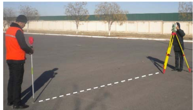
Figure 4. Reference measurements on the selected road segment with total station 06 of Leica Geo-System™.
