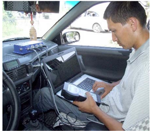
Figure 7. Installation and data collection with roughometer III.
