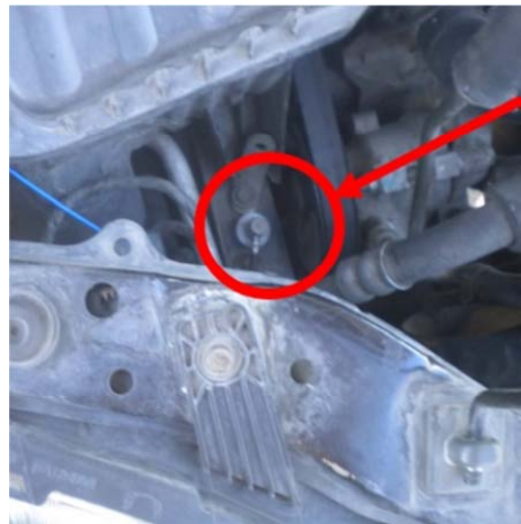
Figure 5. Installation of accelerometers (left side and right side of the axle, and car body) to record road excitations.
