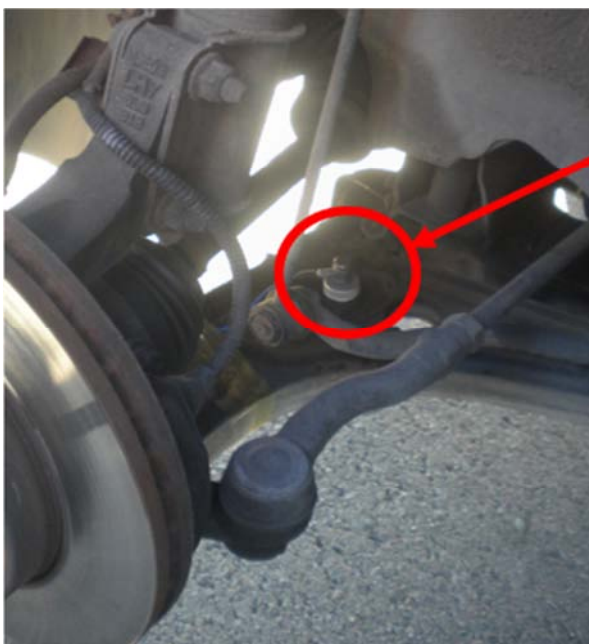
Figure 5. Installation of accelerometers (left side and right side of the axle, and car body) to record road excitations.
